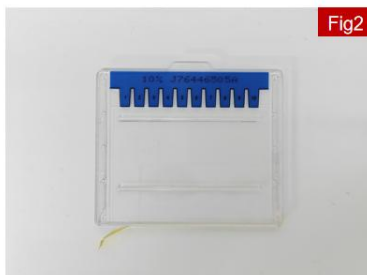
Peel off the sealing tape at the bottom of the gel cassette
