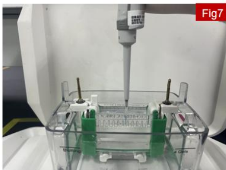
The correct operation for adding samples
