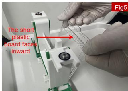
Install the adhesive plate in the core of the electrophoresis tank
