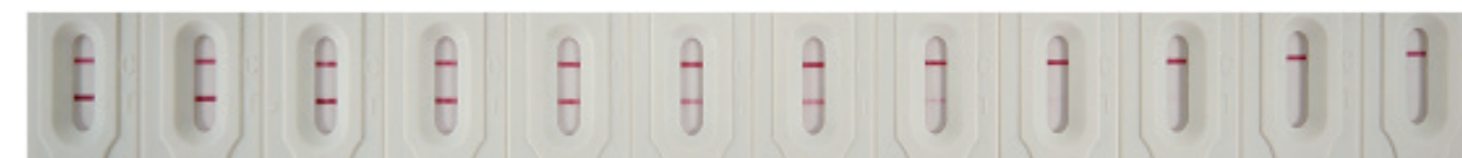
blank 0.3μg/ml 1.6μg/ml 2.5μg/ml 5μg/ml 8μg/ml 10μg/ml 20μg/ml 40μg/ml 40μg/ml 200μg/ml 1mg/ml
